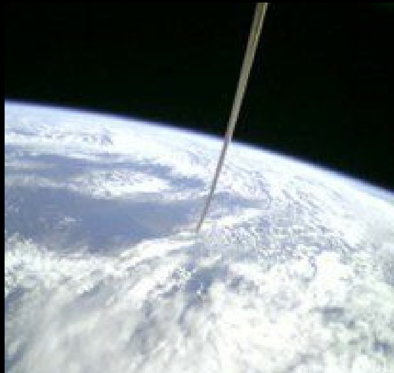
ANTENNA/BOOM ARM MONITORING WITH SELFIECAM
